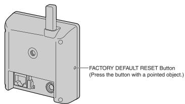
Pressing the FACTORY DEFAULT RESET button resets the camera to factory default. If you lose your user name and password, use this button to reset the camera. To restore the wireless connection, access the camera by using a wired connection and set up the wireless configuration. (For BL-C20A, see Getting Started.)
